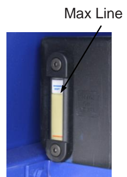
Fig 7.4 Hydraulic Tank Site Gauge
