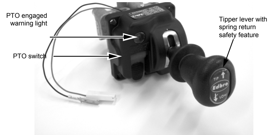
Fig. a. Combined PTO & tipper air controls
