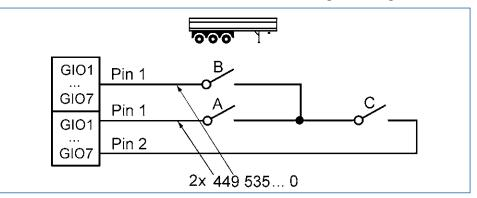
Mechanical switch III for road finishers to positive at analogue TEBS E input
