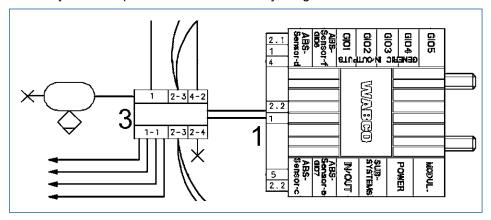
In the absence of a PEM, overload protection must be ensured using a separate relay overload protection valve:
