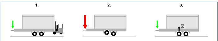
Central axle trailers with an attached forklift are normally constructed so that, when the forklift is attached, the weight distribution is balanced between the front and back. A correspondingly broadly spread support load works as a counterload to the additional weight of the forklift (Fig. 1).
