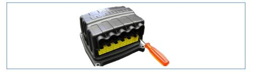
Mount the electronic extension module vertically only, with the cable openings facing the bottom or the side.
