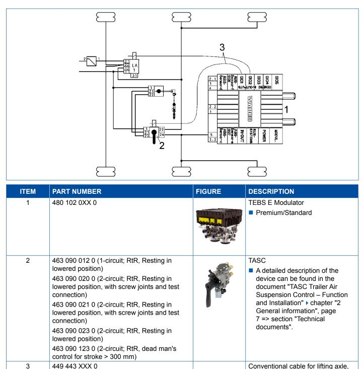
Conventional cable for lifting axle, RtR
