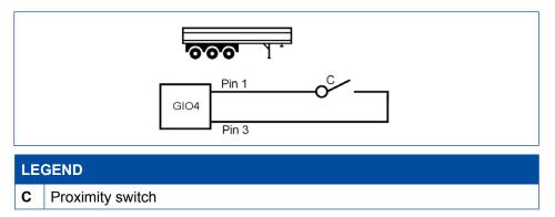
Proximity switch with separate deactivation of the road finisher and unloading level (Figure 2)
