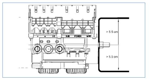
Mount the modulator on a sufficiently sized U-section, angle section, or a suitable reinforced member that is at least 4 mm thick (applies to steel sections).
