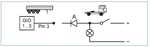
Trailer / signal from towing vehicle - (ground)
