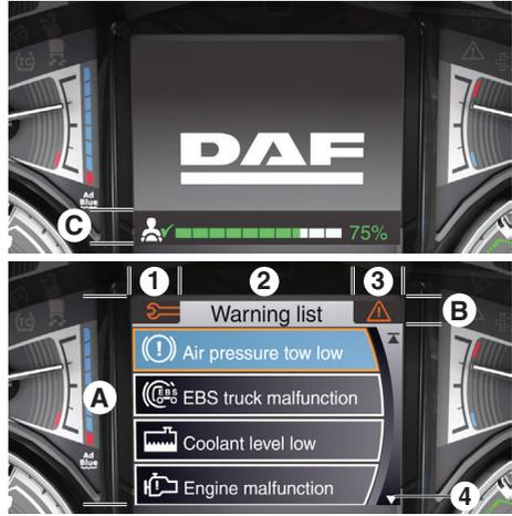
The system is controlled using the Menu Control Switch (MCS). Turn the MCS to select and press to enter a menu, function or setting. Press the Enter key to go back one level or press and hold to exit the menu fully.
