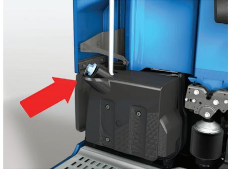
When filling the AdBlue tank and there is (a chance for) frost, fill it to maximum 75%.
