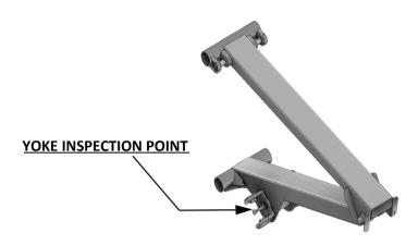
Operators and Service agents are advised to inspect this area during routine maintenance. In extreme cases, a loose bolt can allow the cylinders to move sideways and possibly result in fouling of the chassis frame resulting in cylinder and chassis damage. Inspection and repair should be carried out on a regular basis if necessary.
