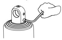
fig e - bleeding an eye-ended hoist
