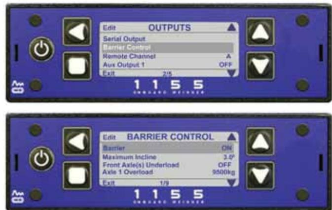
Turn Barrier Control OFF (Outputs – Barrier Control – press EDIT).
