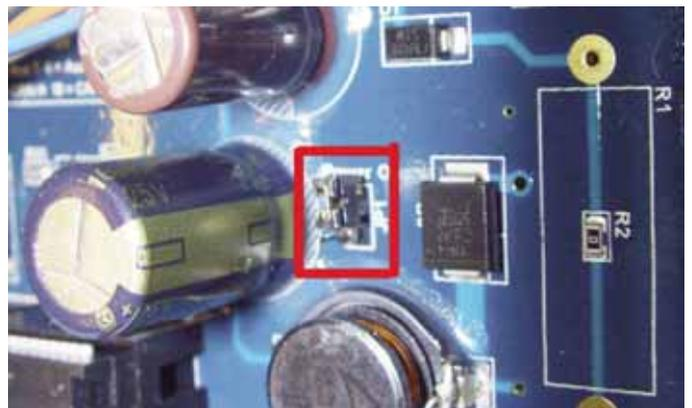
To reset the display to go ON with the ignition, disconnect and remove the display from the vehicle, open the case, remove the jumper and place over BOTH pins - see photograph 3.
