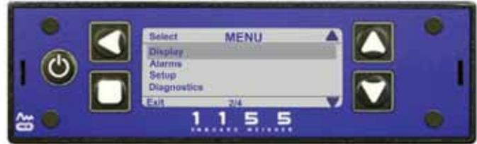
Here you can set the operating mode to Auto or Manual, set the Gross and Net weights at which the alarm will sound and set the Body Up alarm threshold.
