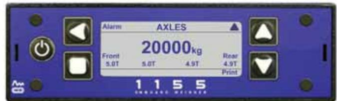
This has the current weight, in Tonnes, shown for each axle.
