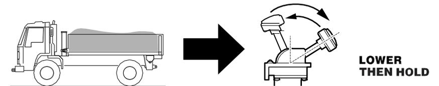
When **LOADING** put the cab control in **LOWER** to ensure that no oil is trapped in the cylinder and the entire load rests on the chassis. Then return the control to **HOLD** when travelling.
