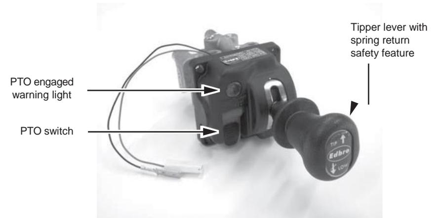
Fig. a. *Combined PTO & tipper air controls*
