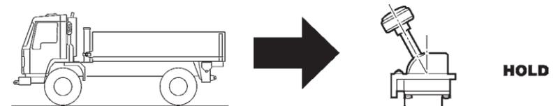
When **UNLADEN** leave the cab control in **HOLD** to minimise body bounce.
