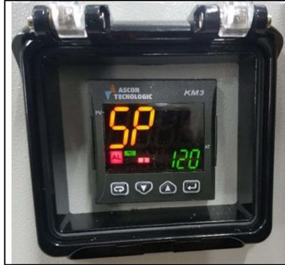
The instrument will automatically go back to its home screen after approximately 20 seconds. Ensure the lid is clipped shut to avoid any damage to control unit.
