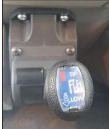
Before any operation of the body is started you must ensure there are no operatives or bystanders close to the vehicle, that there is sufficient height above the tipper and there are no powerlines or obstructions overhead.
