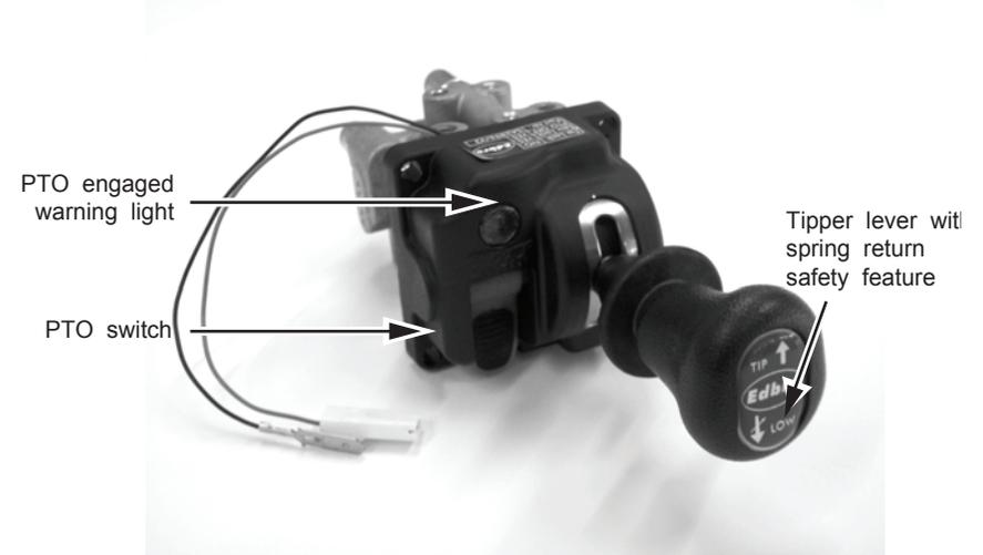
Fig. a. Combined PTO & tipper air control
