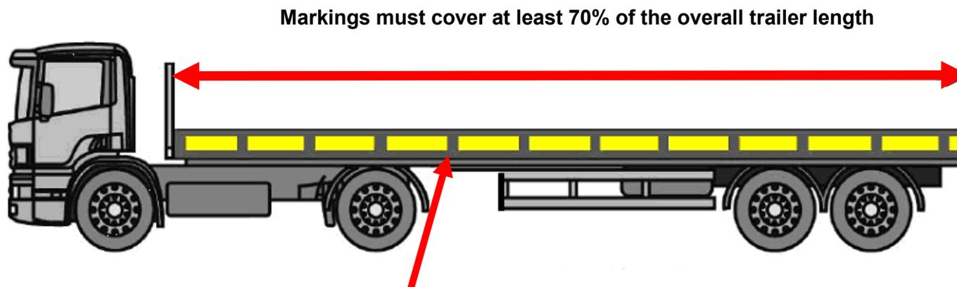
The lowest edge must be between 250mm and 1500mm from the ground. If 1500mm is not practicable this can be increased to 2500mm.
