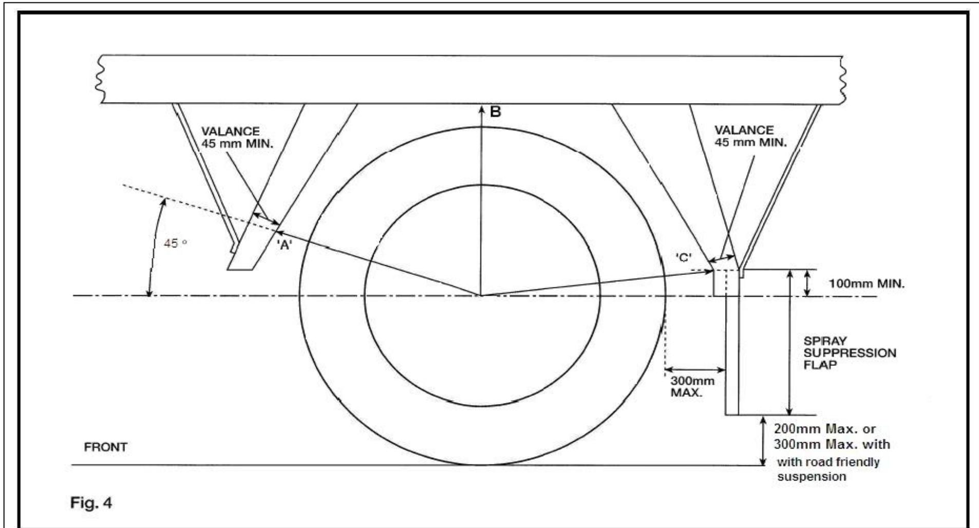
The lower edge of the outer valance shall not exceed 1.8 X tyre radius on steerable wheels, or 1.5 X tyre radius on non-steerable wheels at points A, B & C
